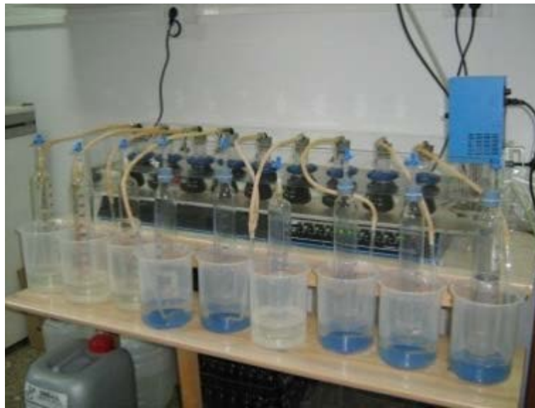
Figure 7: Equipment for Anaerobic digestion in two stages (IG Pilot plant)
